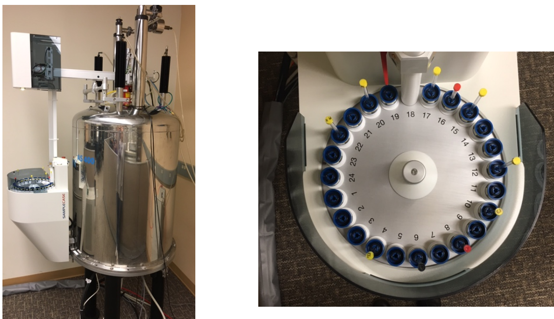
Figure 1: (A) A side view of the Bruker 400 magnet and autosampler. (B) View of the top of the autosampler's carousel showing the 24 sample positions.
