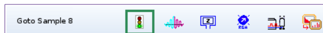
Figure 3: The sample status icon bar that appears on the top right-hand side of the IconNMR screen. Each icon represents a specific spectrometer action being performed on the current sample. When the icon is flashing and is outlined in green, that action is currently in process. When the action is completed, the icon will be outlined in green, but will no longer flash.
