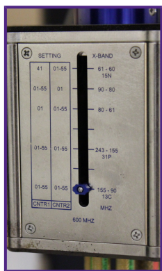
Figure 3.1: The X-BAND indicator on the Inova 600’s NMR probe after adjusting the X-BAND knob to select the ^{13}\text{C} tuning range.
