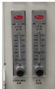
Figure 2. A close-up of the cooling air and VT gas controls located on the spectrometer's magnet leg. In order to perform low-temperature NMR experiments, the VT gas should be increased to 20 LPM. The cooling air should not be increased.
