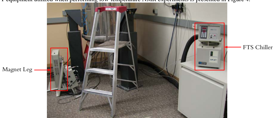
Figure 4. Overview of the VT equipment used when performing low-temperature NMR experiments on the Inova 600.
