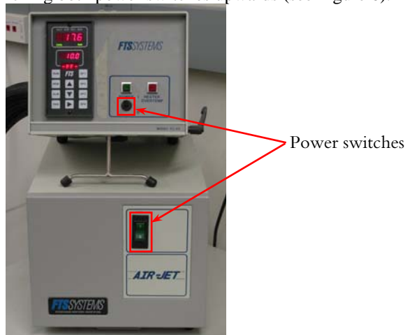
Figure 6. The FTS chiller and its two power switches.
