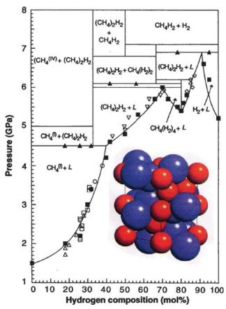
Fig. 8 Pressure-mole fraction diagram of the binary molecular system CH<sub>4</sub>-H<sub>2</sub> at 298 K. Inset: crystal structures of CH<sub>4</sub>(H<sub>2</sub>)<sub>2</sub> compound (space group P6<sub>3</sub>/mmc), blue balls denote CH<sub>4</sub> molecules and red balls denote H<sub>2</sub>. Reproduced with permission.<sup>221</sup> Copyright 1996 AAAS.
