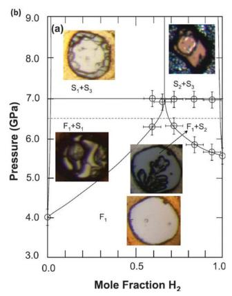
Fig. 10 (a) Crystal structure of  $SiH_4(H_2)_2$  (space group  $F\overline{4}3m$ ). The blue and red balls denote SiH<sub>4</sub> and H<sub>2</sub> molecules respectively. (b) Pressure-mole fraction diagram of the SiH<sub>4</sub>–H<sub>2</sub> binary system. Reproduced with permission. <sup>256</sup> Copyright 2009 American Physical Society.
