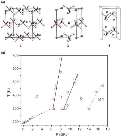
Fig. 4 (a) Crystal structures of NaBH<sub>4</sub>. The space groups for different phases and presentation legends are: 1:  $Fm\bar{3}m$  (α phase); 2:  $P\bar{4}2_1c$  (β phase); 3: Pnma (γ phase), purple: Na, pink: B and white: H. Reproduced with permission.<sup>135</sup> Copyright 2007 American Chemical Society. (b) Pressure–temperature phase diagram of NaBH<sub>4</sub>. Reproduced with permission.<sup>141</sup> Copyright 2009 American Institute of Physics.
