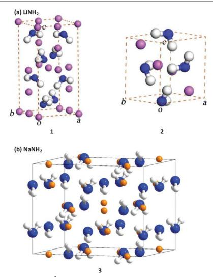
**Fig. 6** Crystal structures of (a) LiNH<sub>2</sub> (1: space group  $I\overline{4}$  (α phase) and 2: space group  $P2_1$  (β phase)), reproduced with permission. Chemical Society; and (b) NaNH<sub>2</sub> (3: space group Fddd). Atom colors: H: white; N: blue; Li: pink; Na: orange.
