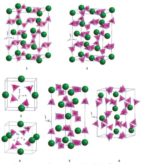
Fig. 5 Crystal structures of Ca(BH<sub>4</sub>)<sub>2</sub>. The space groups for different phases are:  $\alpha$  phase, Fddd (1) or F2dd (2);  $\beta$  phase, P\(\bar{4}\) (3) or P4<sub>2</sub>/m (4);  $\gamma$  phase, Pbca (5);  $\alpha$ ′ phase, /42d (6). Atom colors: H: white; B: pink; Ca: green.
