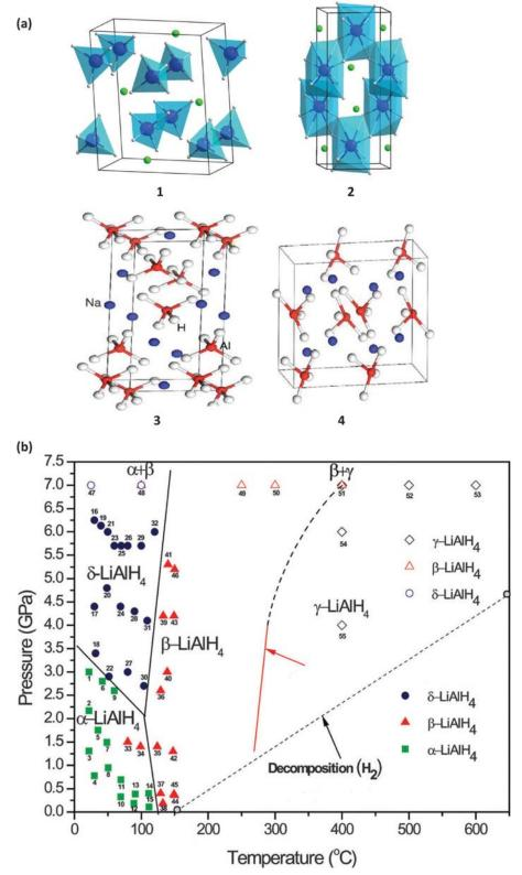
**Fig. 2** (a) Crystal structures of LiAlH<sub>4</sub> (1: space group  $P2_1/c$  (α phase) and **2**: space group I2/b (β phase), atom colors: H: white; Al: blue; Li: green) and NaAlH<sub>4</sub> (3: space group  $I4_1/a$  (α phase) and **4**: space group  $P2_1/c$  (β phase)). (b) Pressure–temperature phase diagram of LiAlH<sub>4</sub>. Reproduced with permission.<sup>104</sup> Copyright 2010 American Chemical Society.
