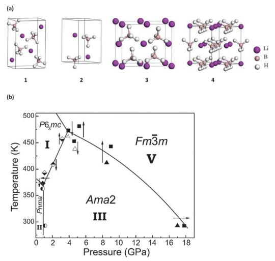
Fig. 3 (a) Crystal structures of LiBH<sub>4</sub>. The space groups for different phases are: 1: Pnma (α or II); 2: P6<sub>3</sub>mc (I); 3: Ama2 (β or III); 4: Fm5̄m (V). Reproduced with permission.<sup>115</sup> Copyright 2011 International Association of Hydrogen Energy. (b) Pressure–temperature phase diagram of LiBH<sub>4</sub>. Reproduced with permission.<sup>120</sup> Copyright 2008 American Physical Society.
