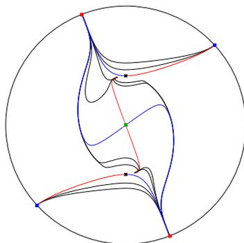
Fig. 2. Phase portrait of system (2.8) for  $B_{21} = 0, A_{21} = B_{12} = A_{12} = A_{30} = 1, B_{30} = 2$ , showing that  $(0, \pm 1)$  are saddle-node nilpotent singular points.
