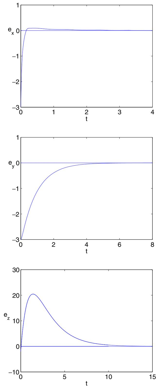
Fig. 4. Time history of the error system (32) for  $c = 4$  using the control law given in Theorem 8, with the initial conditions,  $x_d(0) = -2$ ,  $y_d(0) = -1$ ,  $z_d(0) = 1$ , and  $x_r(0) = 1$ ,  $y_r(0) = 2$ ,  $z_r(0) = 3$ , when  $\delta_x = 0.5$ ,  $\delta_z = 0.5$  and  $\hat{\alpha} = 12$ .
