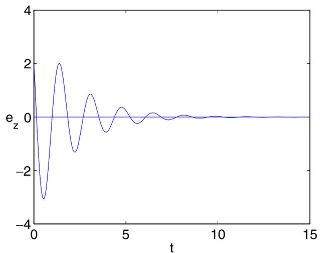
Fig. 5. Time history of the error system (32) for  $c = 4$  using the control law given in Theorem 11, with the initial conditions:  $x_d(0) = -2$ ,  $y_d(0) = -1$ ,  $z_d(0) = 1$ , and  $x_r(0) = 1$ ,  $y_r(0) = 2$ ,  $z_r(0) = -2$ , when  $\delta_x = 0.5$ .
