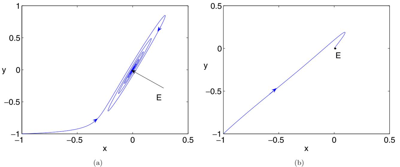
Fig. 2. (a) Trajectory of a five-scroll chaotic attractor for system (1) using the control law given in Theorem 3 for  $k = 1.2$  with the initial condition  $x(0) = -1, y(0) = -1, z(0) = 1$ , convergent to the equilibrium point  $E: (0, 0, 0)$ ; (b) trajectory of a five-scroll chaotic attractor for system (1) using the control law given in Theorem 4 for  $k_1 = k_2 = 1$  with the initial condition  $x(0) = -1, y(0) = -1, z(0) = 1$ , convergent to the equilibrium point  $E: (0, 0, 0)$ .
