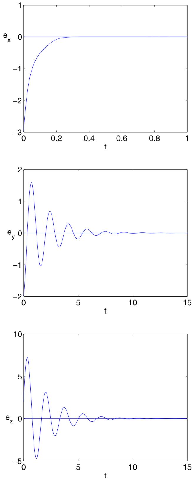
Fig. 3. Time history of the error system (32) for  $c = 4$  using the control law given in Theorem 7, with the initial conditions:  $x_d(0) = -2$ ,  $y_d(0) = -1$ ,  $z_d(0) = 1$ , and  $x_r(0) = 1$ ,  $y_r(0) = 1$ ,  $z_r(0) = -1$ , when  $\delta_x = 0.5$ .
