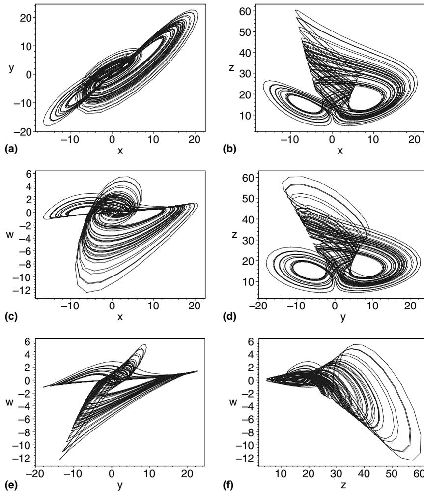
Fig. 3. Simulated phase portraits of the hyperchaotic system (2.1) with parameter values  $a = 37, b = 3, c = 26, d = 38$ , projected on (a) the  $x$ - $y$  plane; (b) the  $x$ - $z$  plane; (c) the  $x$ - $w$  plane; (d) the  $y$ - $z$  plane; (e) the  $y$ - $w$  plane; and (f) the  $z$ - $w$  plane.
