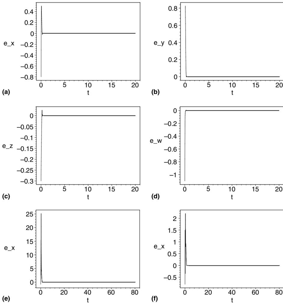
Fig. 6. Simulated results for the hyperchaotic system (2.1) with parameter values  $a = 37$ ,  $b = 3$ ,  $c = 26$ ,  $d = 38$ : (a)–(d) the time histories of the error signals  $e_x$ ,  $e_y$ ,  $e_z$  and  $e_w$  under the controller given in Case (i) of Theorem 1 with  $k_2 = 30$ ,  $k_3 = 40$ ; (e) and (f) the time histories of the error signals  $e_x$  under the controller given in Case (i) of Theorem 1 with the control gains (e)  $k_2 = 6$ ,  $k_3 = 8$ , and (f)  $k_2 = 15$ ,  $k_3 = 0$ .
