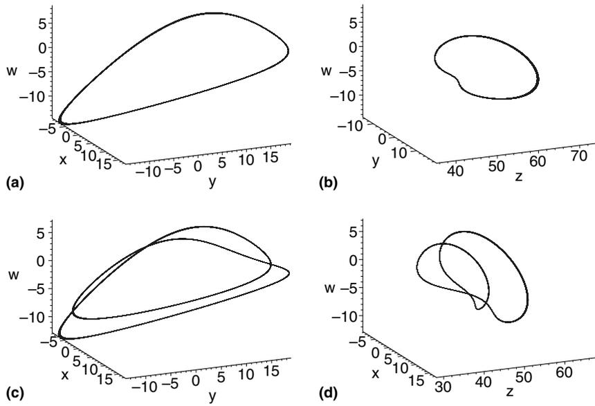
Fig. 4. Simulated limit cycles for the hyperchaotic system (2.1) with parameter values  $a = 37, b = 3, d = 38$ : (a) and (b) a single limit cycle when  $c = 33.6$ ; (c) and (d) a double limit cycle when  $c = 32.6$ .
