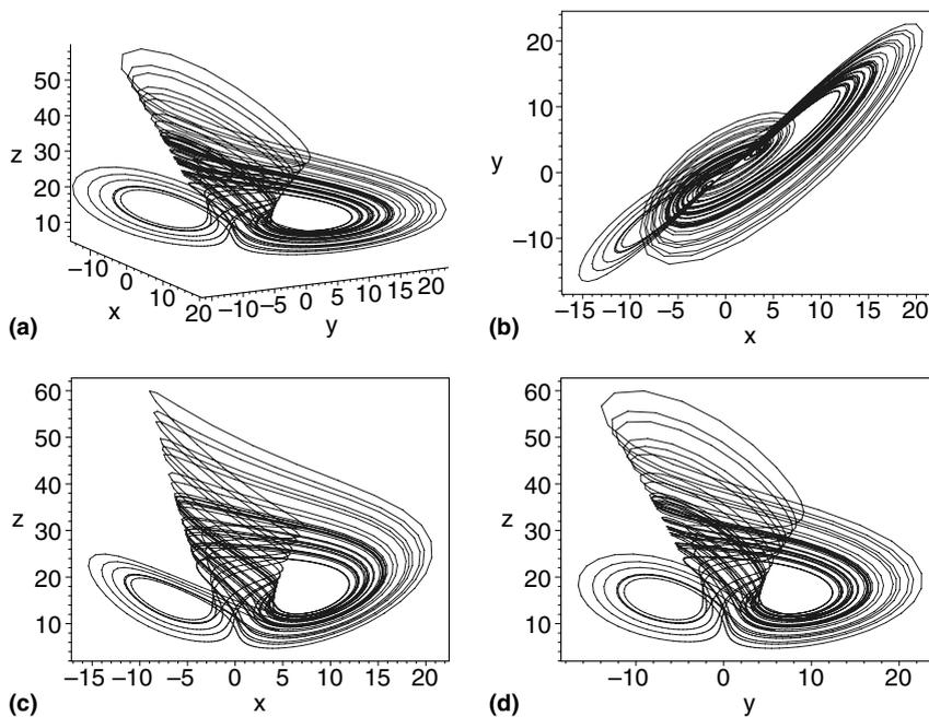
Fig. 5. Simulated phase portraits of the chaotic system (2.2) with parameter values  $a = 37, b = 3, c = 26$ , projected on (a) the  $y$ - $z$  space; (b) the  $x$ - $y$  plane; (c) the  $x$ - $z$  plane; and (d) the  $y$ - $z$  plane.
