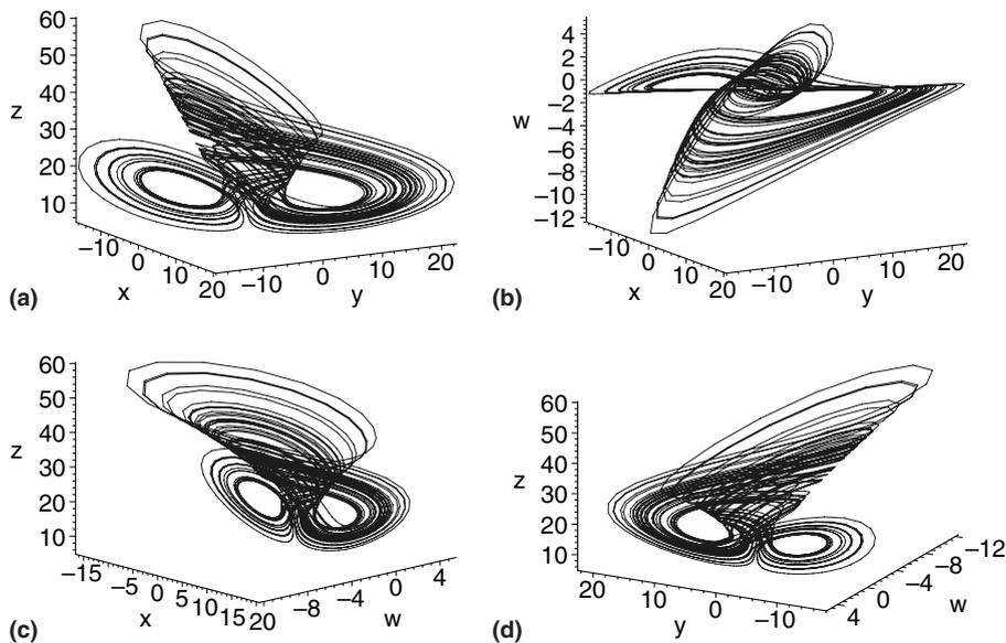
Fig. 2. Simulated phase portraits of the hyperchaotic system (2.1) with parameter values  $a = 37, b = 3, c = 26, d = 38$ , projected in (a) the  $x$ - $y$ - $z$  space; (b) the  $x$ - $y$ - $w$  space; (c) the  $x$ - $z$ - $w$  space; and (d) the  $y$ - $z$ - $w$  space.
