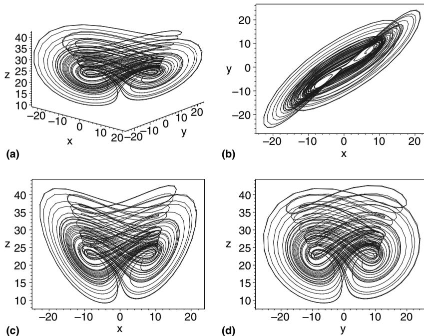
Fig. 1. Simulated phase portraits of the Chen system (1.3) with parameter values  $a = 35$ ,  $b = 3$ ,  $c = 28$ , projected (a) in the  $x$ - $y$ - $z$  space; (b) on the  $x$ - $y$  plane; (c) on the  $x$ - $z$  plane; and (d) on the  $y$ - $z$  plane.
