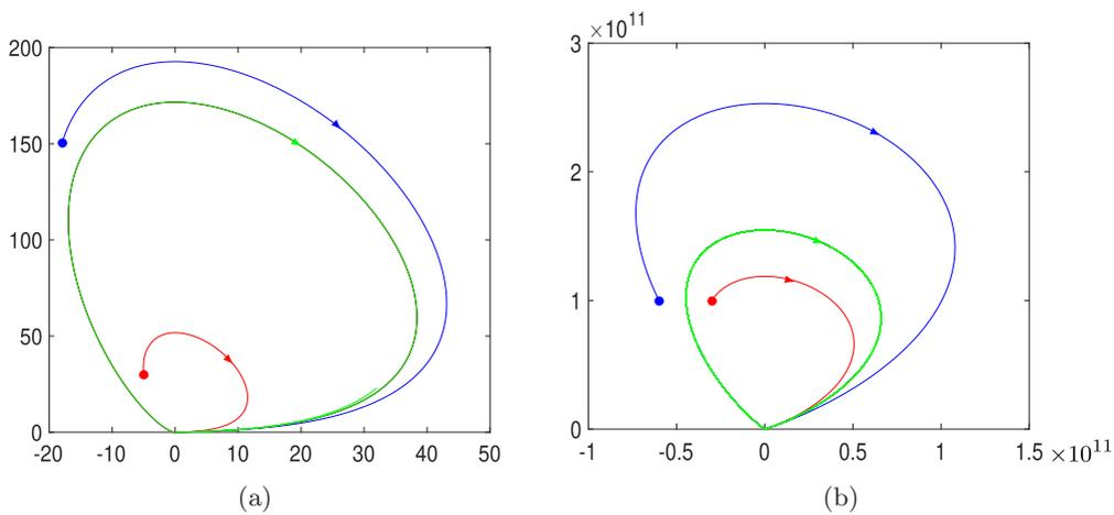
Fig. 4. Simulation of the stable big limit cycle using Matlab solver ODE23: (a) for system (10) taking  $\lambda = -2 \times 10^{-8}$ ,  $\epsilon = -0.001$ ,  $\delta = -0.1$ , with initial points  $(-18, 150)$  and  $(-5, 30)$ ; and (b) for system (10) taking  $\delta_1 = 0.01$ ,  $\delta_2 = 0.00002$ , with initial points  $(-0.6 \times 10^{11}, 10^{11})$  and  $(-0.3 \times 10^{11}, 10^{11})$ .
