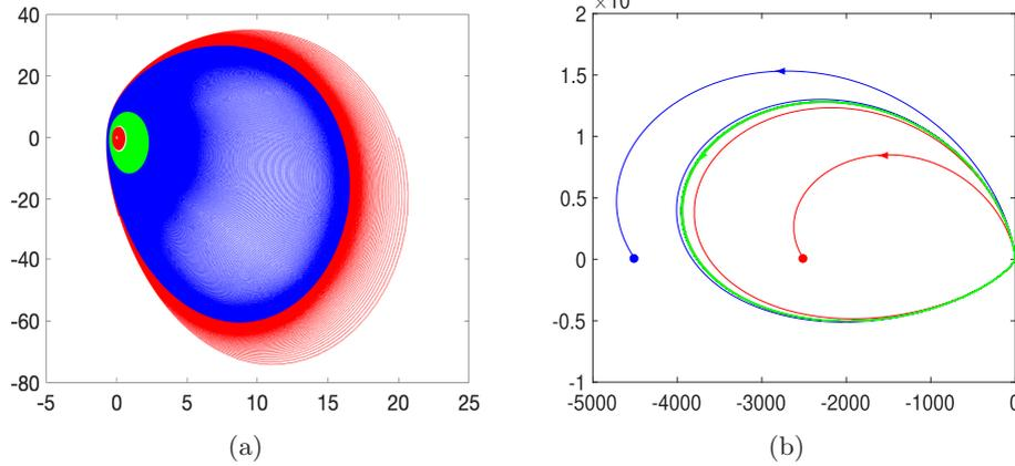
Fig. 6. Simulation of limit cycles using Matlab solver ODE23 for system (8) with the parameter values given in (17): (a) three limit cycles around the unstable focus  $(0, 0)$ ; and (b) one big unstable limit cycle (in green color) around the stable focus  $(-6.2596, 7.4498)$ , with two trajectories starting from the initial points  $(-4500, 0)$  (in blue color) and  $(-2500, 0)$  (in red color).
