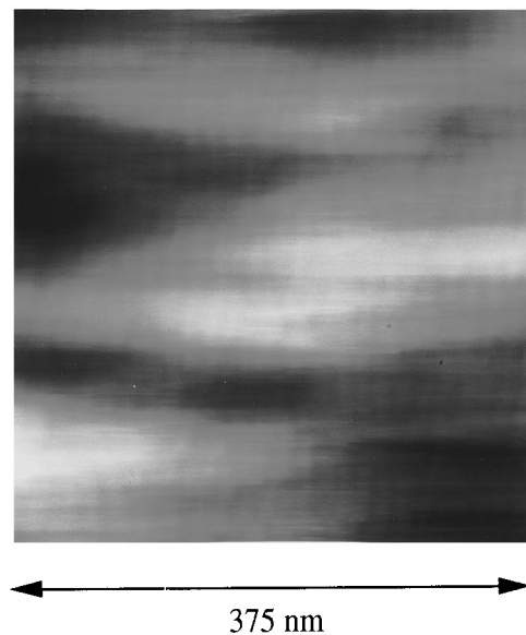
FIG. 2. Topography of PEO surface imaged with small forces of 6 nN after the large-force scanning of 50 nN. The gray scale level is 0–30 nm. There are stripes perpendicular to the large-force scanning direction.
