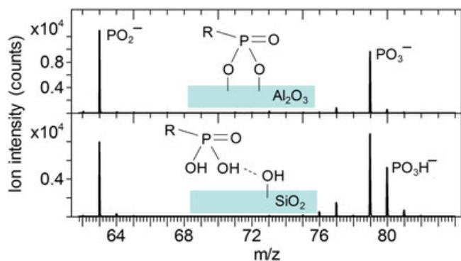
**Figure 2.** Secondary negative ion mass spectra of octadecylphosphonic acid (OPA) self-assembled monolayers on Al and Si oxides. The bonding modes of OPA molecules with the 2 different substrates are also depicted.
